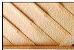
Ribs Notched into Liner for Soundboard Crown Retention
