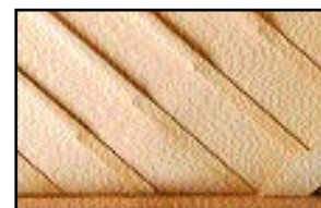
Ribs Notched into Liner for Soundboard Crown Retention
